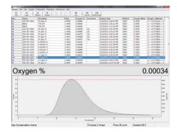
System interface incorporates sample information, sample results, statistics, and system controls.
